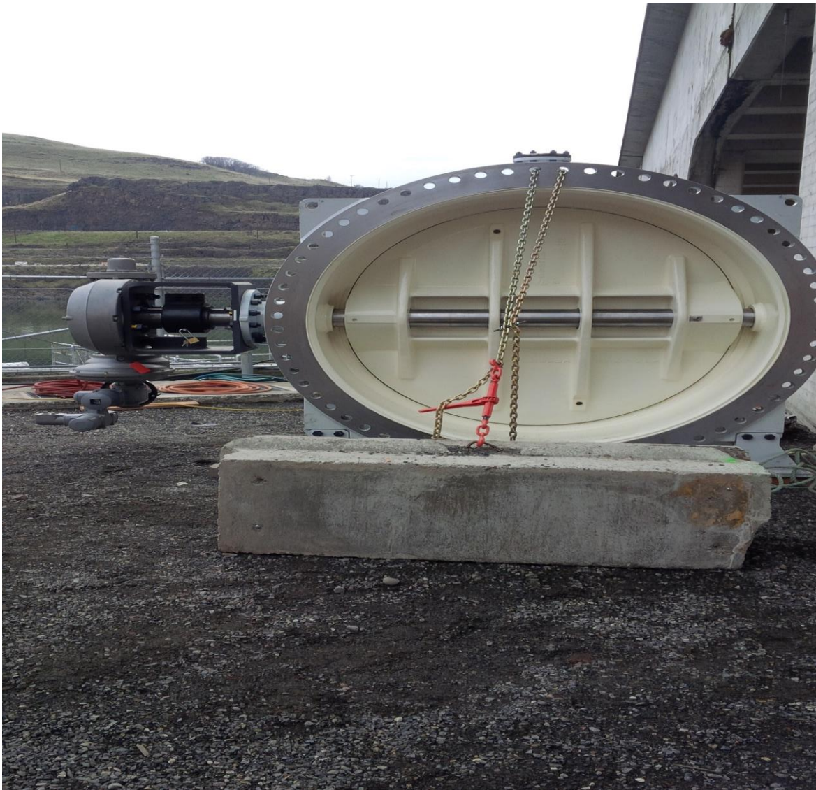
New italian 7' valve ready for install
